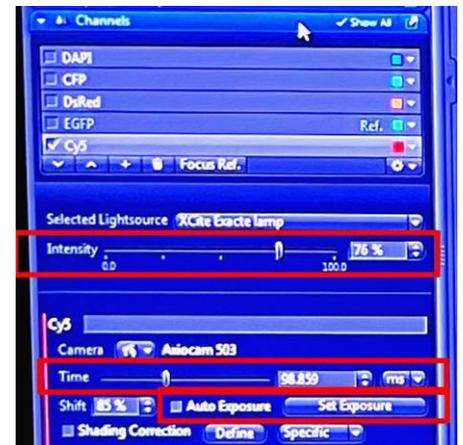
Fig 8. Channels Module. Set intensity and exposure time
