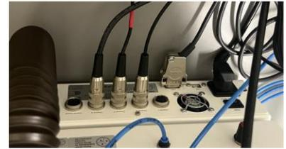
Fig 4. Back panel heater connections
