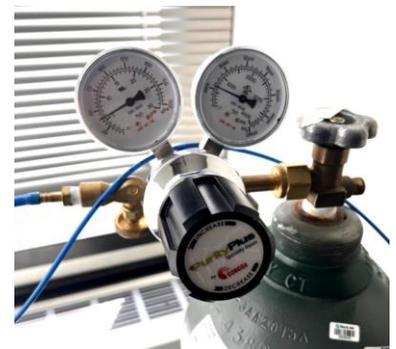
Fig 7. CO2 regulator, main valve (gray), and tank
